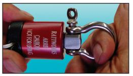
Grasp body and base assembly and firmly pull toggle as shown twisting and turning. If by chance it comes apart repeat steps 2, 3, 4, 5, 8 and 9. After use, clean all parts with gun solvent and relubricate o-rings with silicon grease and
