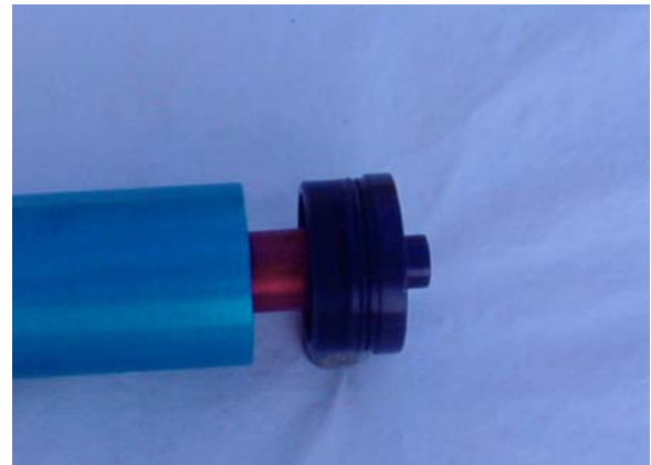
STEP 18: SLIDE FORWARD CLOSURE ONTO EXPOSED FUEL TANK. PUSH ASSEMBLY INTO MOTOR TUBE.
