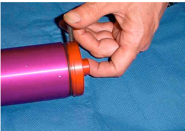
STEP 19: APPLY KRYTOX TO O-RING. THREAD FORWARD CLOSURE INTO MOTOR TUBE, USE 10-32 SOCKET SCREW TO AID IN TIGHTING.
