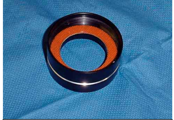
STEP 16: PLACE NOZZLE INSULATOR RING INTO REAR CLOSURE.
