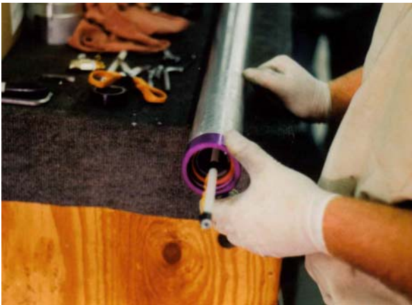
STEP 17: THREAD REAR CLOSURE ONTO MOTOR TUBE.
