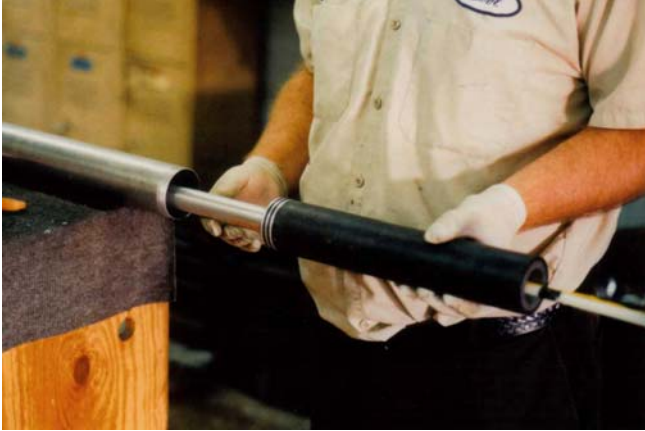
STEP 15: SLIDE FUEL TANK COMBUSTION CHAMBER ASSEMBLY INTO MOTOR TUBE. PUSH ASSEMBLY AT LEAST 1" PAST LIP.
