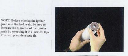
Step 3: Press ignitor grain into plastic fuel grain as shown.
