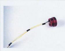
Step 2: Tape Firestar electric ignitor to filling line as shown.
