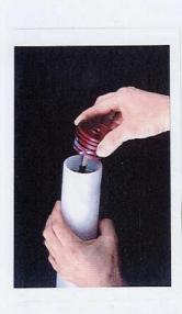
Press injector assembly into top of fuel grain, ensure lower half of injector is completely in fuel grain.
