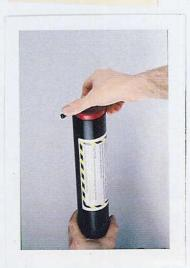
Step 7: Thread forward bulkhead into top of motor case, use 1/4-20 cap screw by threading into vent hole, tighten bulkhead all the way.
