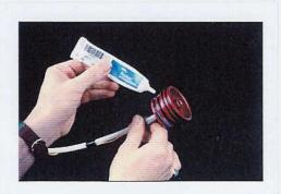
Step 4: Lubricate O-rings on injector with krytox grease. Feed fill line and electric ignitor wires through top of fuel grain and out the nozzle.
